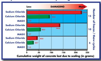
Per SHRP H-205.8 Test Method Using 3% Brine Solution
